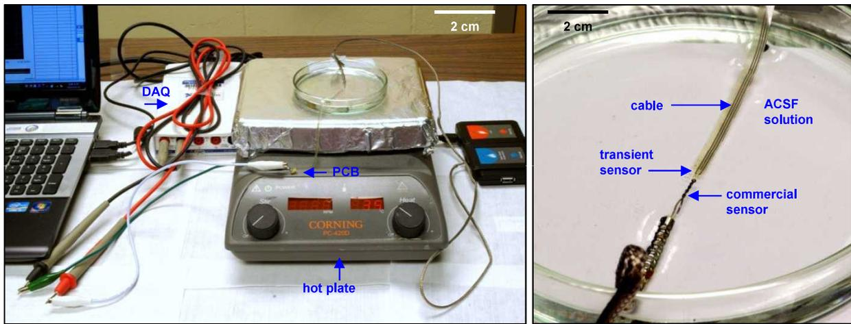
**Figure S13.** In vitro setup for transient temperature sensors.
