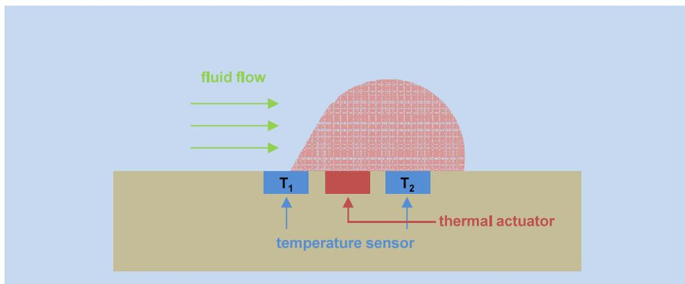
**Figure S14.** Principle of flow rate monitor based on a thermal actuator and a pair of temperature sensors. The difference between the temperatures recorded at the two temperature sensors ( $T_2 - T_1$ ) increases as the flow rate increase.
