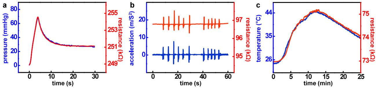
**Figure S10.** Calibration of resistance change to a) pressure, b) acceleration, and c) temperature.
