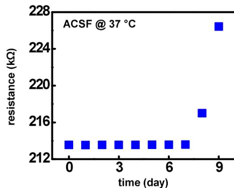
**Figure S28.** Resistance measurement of a pressure sensor with polyanhydride encapsulation with constant external pressure.
