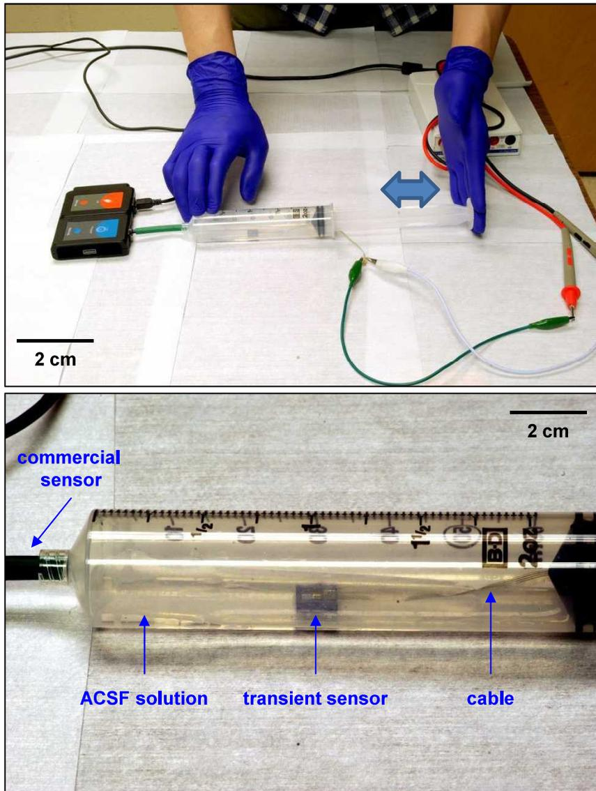
**Figure S9.** In vitro test of transient pressure sensor in ACSF solution.
