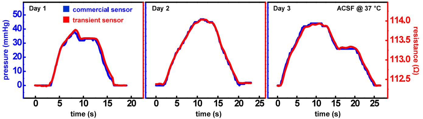
**Figure S26.** In vitro operation of bioresorbable pressure sensor with functional lifetime controlled with a biodegradable encapsulation layer.
