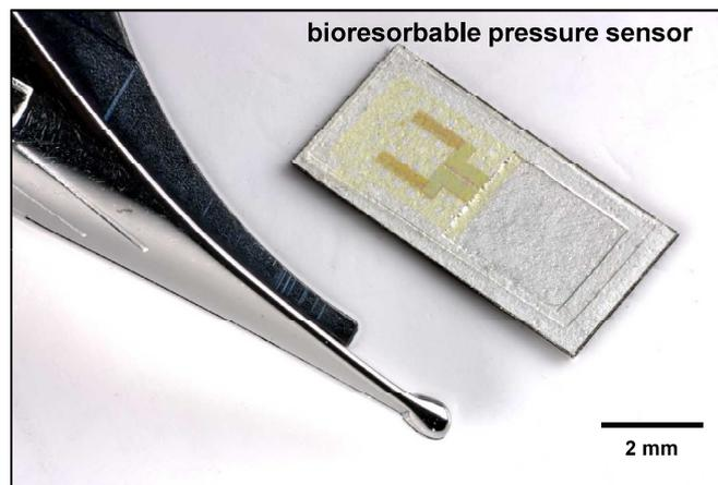
**Figure S3.** Biodegradable pressure sensor with Mg trench structure. Trench depth and thickness of Mg foil are  $\sim 40 \mu\text{m}$  and  $\sim 80 \mu\text{m}$ , respectively.
