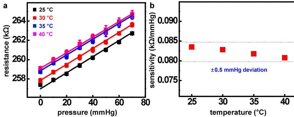
**Figure S19.** Calibration of the temperature dependent piezoresistivity. a) Resistivity variation to applied pressure at various temperatures (error bars represents standard deviation). b) Variation of sensitivity of resistivity to pressure associated with changes in temperatures. The change of piezoresistivity sensitivity is negligible across the expected range of brain temperatures.
