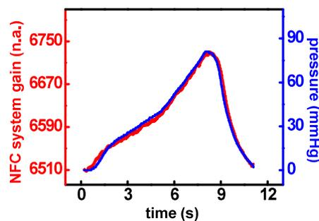
**Figure S37.** Response of a commercial pressure sensor (blue) and a wireless, biodegradable system (red) to time-varying pressure over a range relevant to intracranial monitoring.
