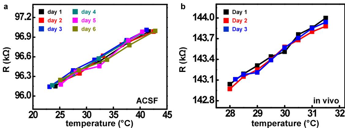
**Figure S29. In vitro and in vivo demonstrations of biodegradable temperature sensors.** a) Calibration curves for resistance to temperature indicate stable operation over 6 days in ACSF. b) Stable in vivo operation was demonstrated for three days. Sensors were encapsulated with a 120 μm thick layer of polyanhydride.
