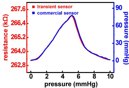
**Figure S8.** Calibration curve of pressure sensor with 2 mm × 2.4 mm × 40 μm dimension.
