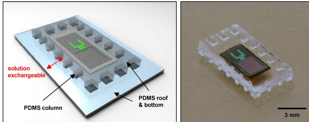
**Figure S17.** Schematic diagram (left) and image (right) of PDMS structure used as a simple mimic of the intracranial space.
