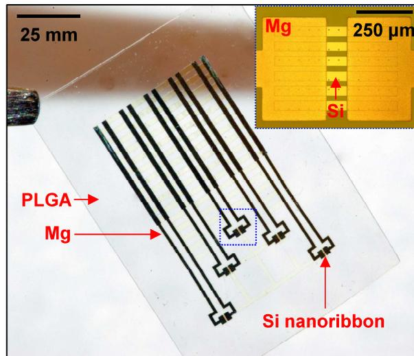
**Figure S15.** Bioresorbable pH sensor constructed with Si-NRs, Mg electrodes and PLGA substrates.
