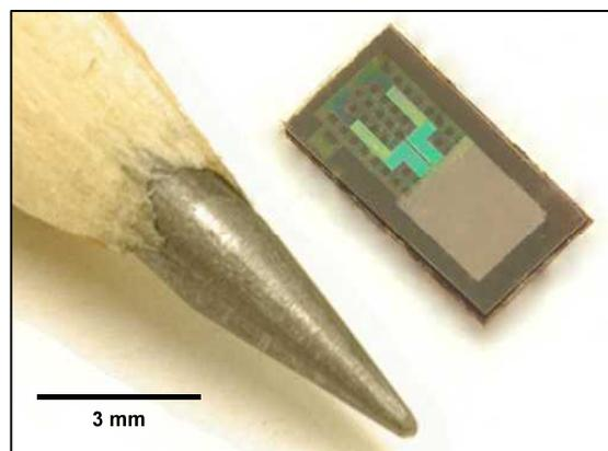
**Figure S4.** Image of a bioresorbable pressure sensor, with a thickness of  $\sim 110 \mu\text{m}$ , a weight of  $\sim 1 \text{ mg}$  and overall lateral dimensions of  $3 \text{ mm} \times 6 \text{ mm}$  and trench dimensions of  $2 \text{ mm} \times 2.4 \text{ mm} \times 40 \mu\text{m}$ .
