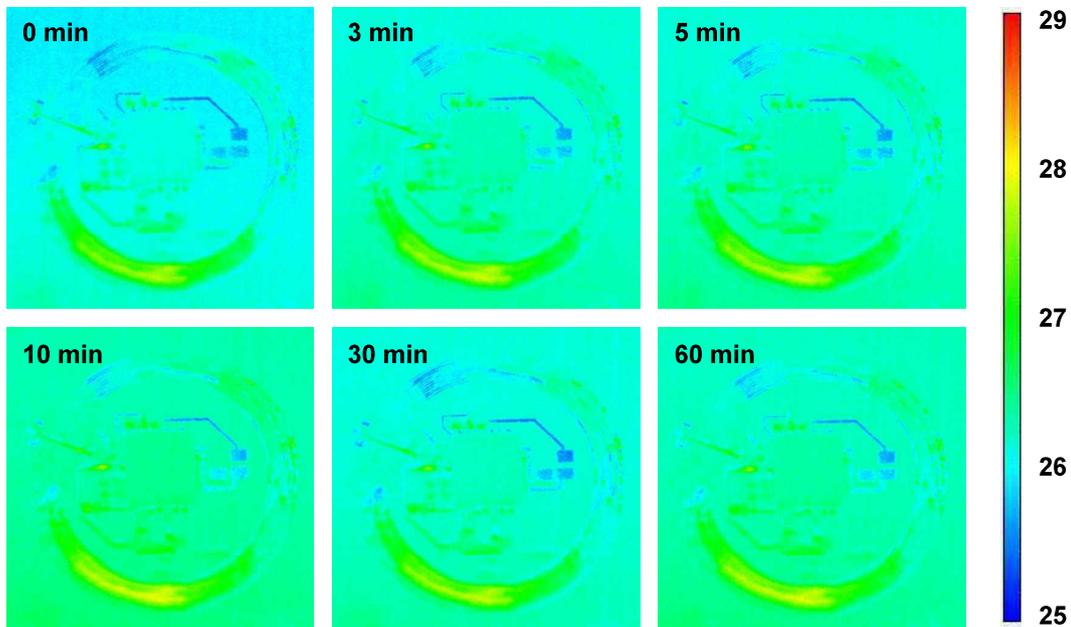
**Figure S33.** IR thermography of an NFC system during wireless operation in air.
