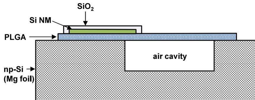
**Figure S1.** Cross-sectional side view of the bioresorbable pressure sensor.
