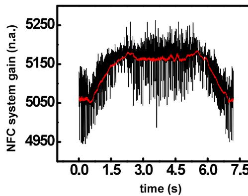
**Figure S36.** Comparison of filtered (red) and unfiltered (black) gain during pressure measurement. Two channels were measurement through NFC system at the same time. The filter function was loaded and performed in the chip.
