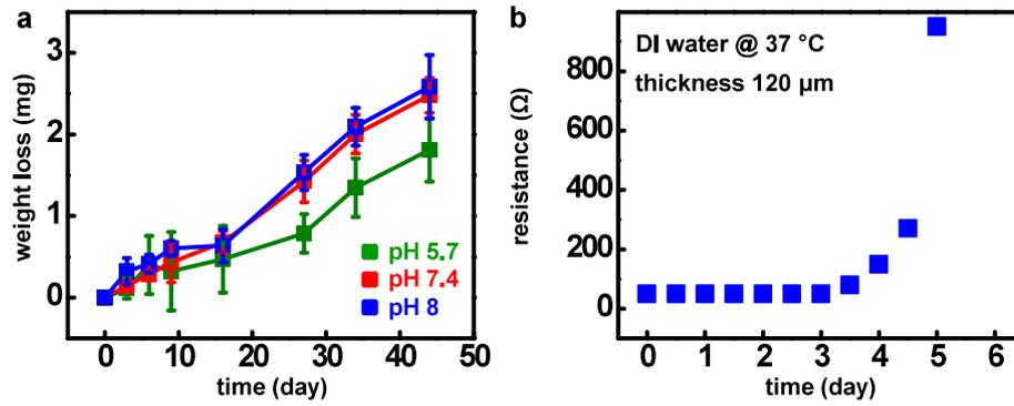
**Figure S24.** a) Dissolution kinetics and b) water permeability (tested by 300 nm thick Mg resistor) of polyanhydride encapsulation.
