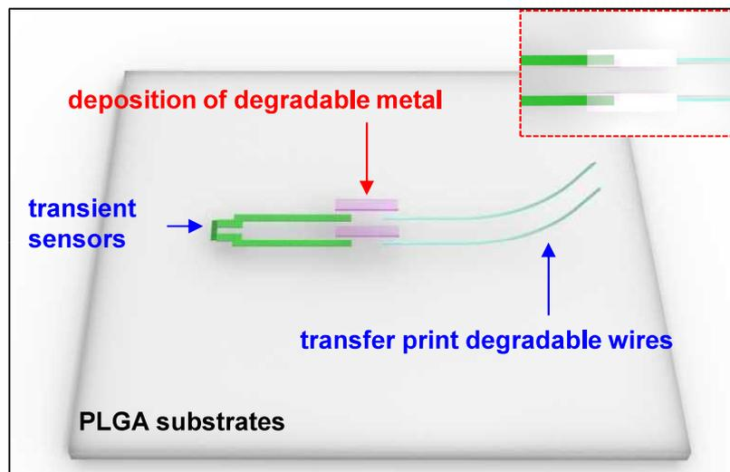
**Figure S20.** Strategy for interconnection between a bioresorbable device and degradable external wires on biodegradable polymer. Transfer printing the biodegradable wires (Mg or Mo) on the biodegradable polymer substrate (PLGA), and depositing dissolvable metal (Mo) between the wires and sensors yield the fully bioresorbable interface.
