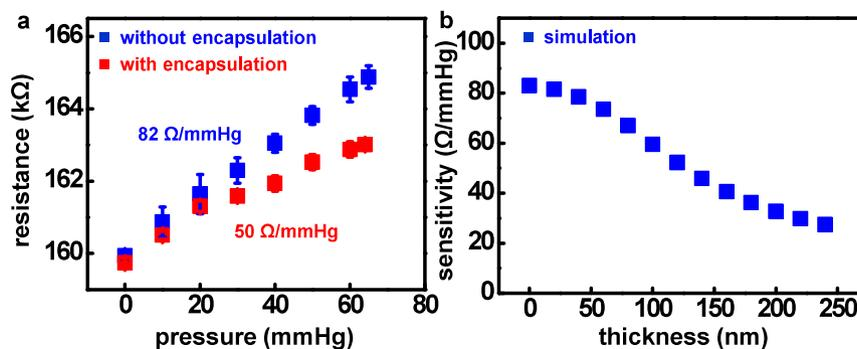
**Figure S22.** Effect of polyanhydride encapsulation on the response of the pressure sensor. a) Calibration curves before and after encapsulation. The calibration factor changes from 82 to 50  $\Omega/\text{mmHg}$  with 120  $\mu\text{m}$  thick encapsulation (error bars represents standard deviation). b) The thickness dependent sensitivity simulated by FEM.
