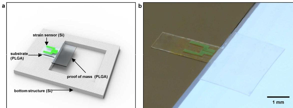
**Figure S11.** Transient accelerometer with Si-NM piezoresistive strain sensor. a) Materials and structure of accelerometer with PLGA proof mass. b) Image of bioresorbable accelerometer on the Si structure.
