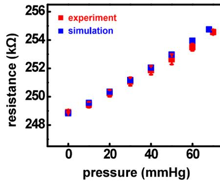
**Figure S7.** Piezoresistive response of the pressure sensor compared to finite element method (FEM) simulation (error bars represents standard deviations).
