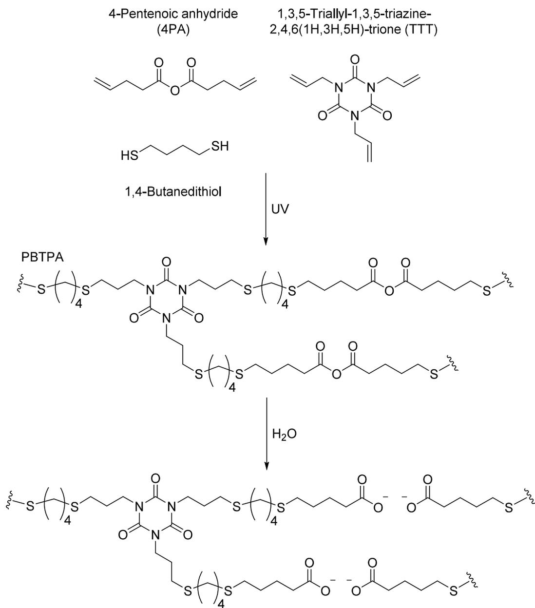
**Figure S23.** Chemistry of synthesis and hydrolysis of a biodegradable polymer (class of polyanhydride) for encapsulation.
