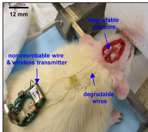
**Figure S21.** Image of the interface between the bioresorbable wires and the wireless transmitter.
