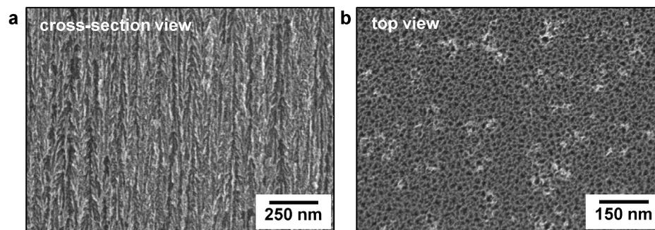
**Figure S2. Scanning electron microscope (SEM) images of nanoporous Si.** a) Cross-section view and b) top view of np-Si structure with ~71 % porosity.
