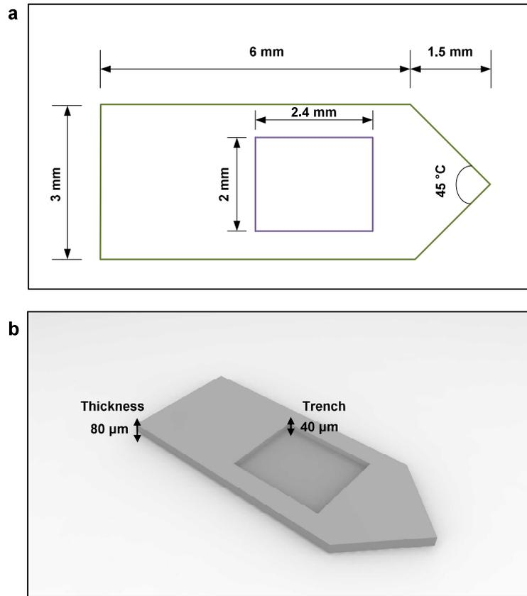
**Figure S38. Geometry of needle substrates of pressure sensor.** a) Lateral geometry and b) three dimensional geometry of Mg needle substrates.
