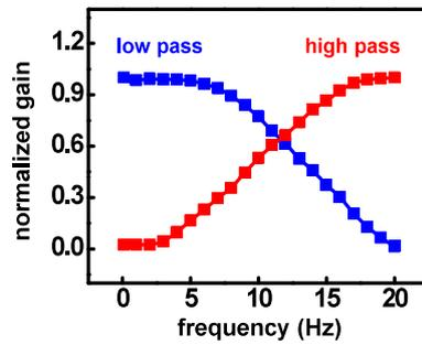
**Figure S35.** Gain response of programmed real-time high (red) and low (blue) pass filtering, performed by the NFC chip, as a function of frequency.
