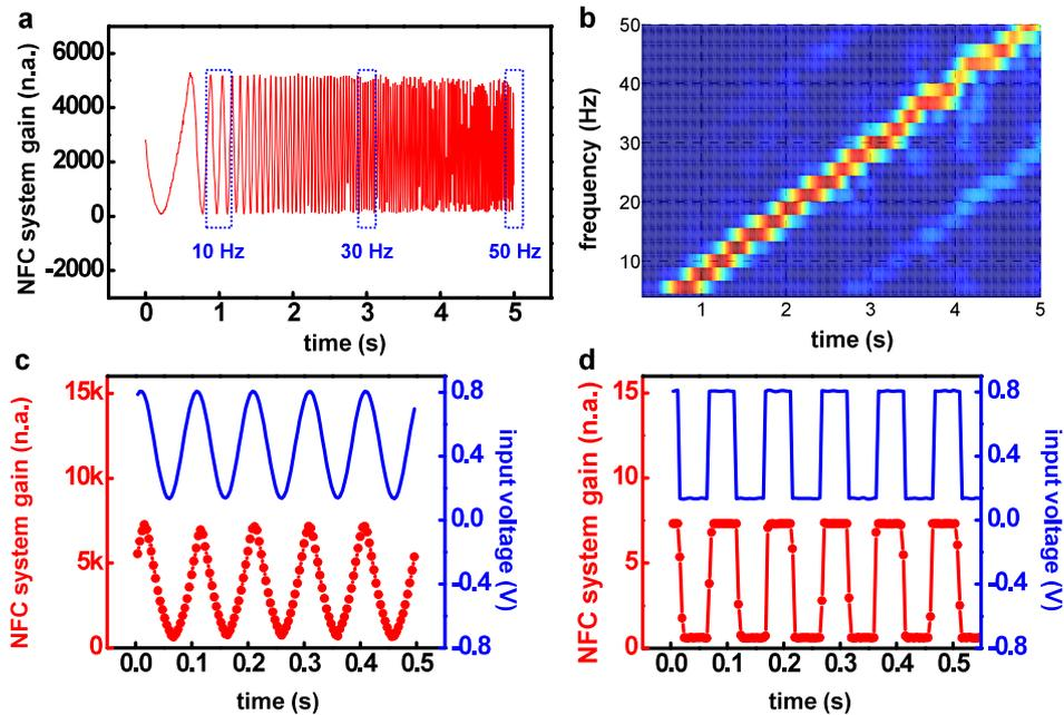
**Figure S34. High sampling rate of NFC system.** a) Wirelessly transmitted voltage sine waves with frequencies between 1 to 50 Hz. Maximum sampling rate of this system is 250 Hz. b) Spectrogram of swept sine wave in Figure 2f. High speed data acquisition of NFC system demonstrated with c) sine and d) square wave of 10 Hz frequency. (Red dot line is the data point measured by NFC system and blue line is input signal from signal generator.)
