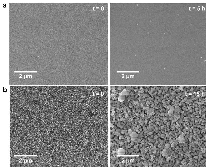
**Figure S18.** Scanning electron microscope (SEM) images of a) Si NMs and b) np-Si at the different stages of dissolution in buffer solution with pH 12 at 37 °C.
