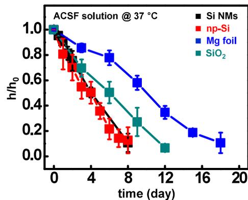
**Figure S16.** Hydrolysis kinetics of materials used in the bioresorbable pressure sensors. Normalized thickness ( $h/h_0$ ) as a function of time during dissolution of individual materials in artificial cerebrospinal fluid (ACSF) at physiological temperature (37 °C). The initial thicknesses were 200 nm for Si nanomembranes (Si NMs), 80 μm for porous Si (p-Si), 80 μm for Mg foil, and 100 nm for SiO<sub>2</sub>.
