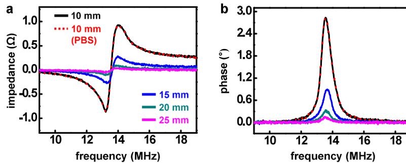
**Figure S32.** Frequency dependent a) impedance and b) phase of the NFC system at the different distance (black line; 10 mm, red dot; 10 mm with 2 mm barrier of phosphate buffer solution (PBS), blue line; 15 mm, cyan line; 20 mm, magenta line; 25 mm).
