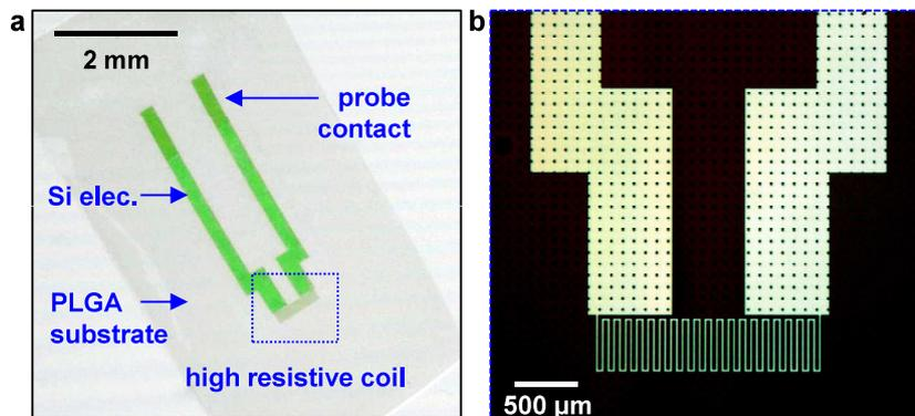
**Figure S12.** Bioresorbable temperature sensor on a thin PLGA film. a) Materials and structure of a thermoresistive Si temperature sensor. b) Microscope image of a dense serpentine Si-NM structure for enhanced thermoresistive response.
