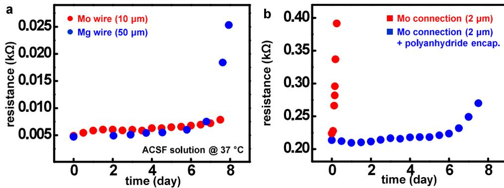
**Figure S27.** Effect of dissolution of metal wires and interconnects on the resistance.
