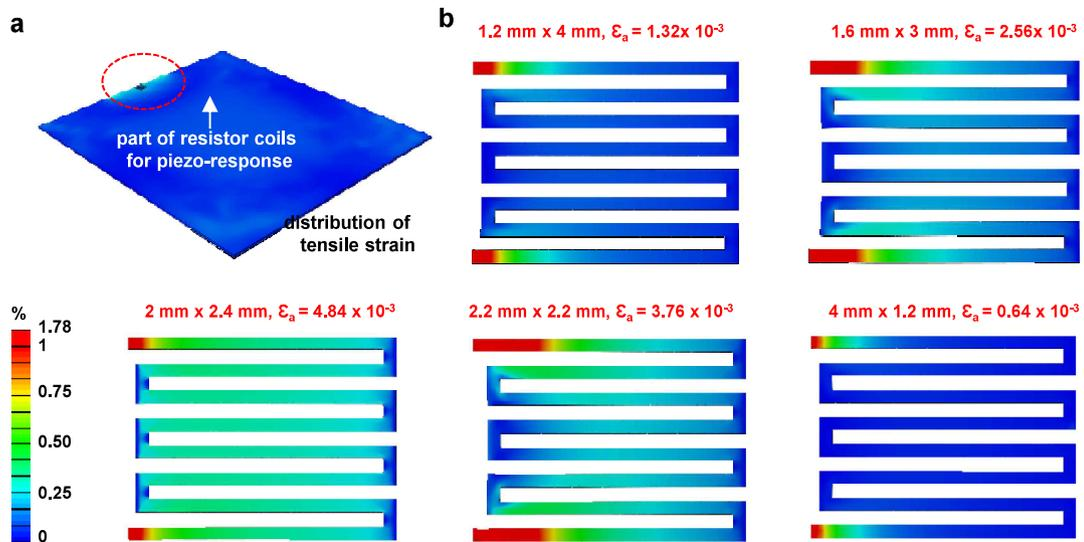
Figure S6. Optimization of trench geometry through stress-strain analysis using the finite element method (FEM). a) Full image of simulated dimension. b) Principle strain distribution around the piezoresistive serpentine sensors for various trench geometries.  $\epsilon_a$  represents average strain on coils.
