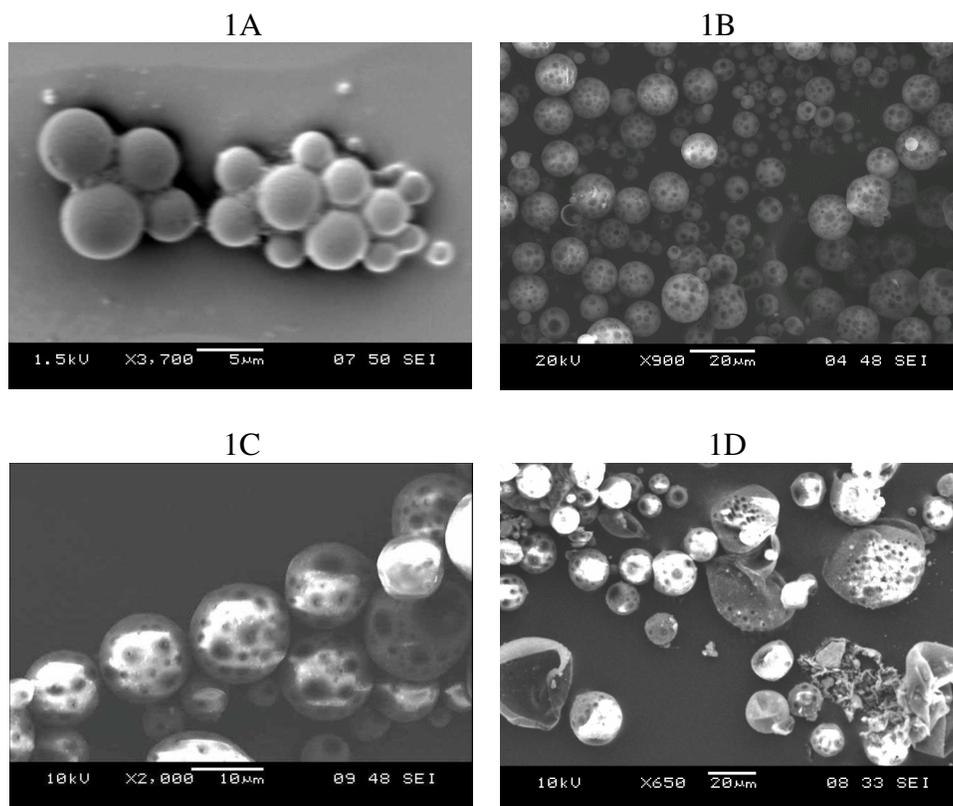
**Figure 1.** SEM image of Humulin R-encapsulated, magnetite PLGA MP. Magnetite content in weight percentage: A) 0%, B) 2%, C) 5%, D) 10%.
