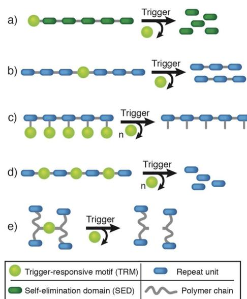
**Figure 2.** Schematic illustration for different trigger-responsive cleavable polymers with trigger-responsive moiety located at (a) terminal, (b) chain center or junction, (c) side chain, (d) main chain, and (e) cross-linked point of polymeric materials and their degradation processes after trigger treatment.
