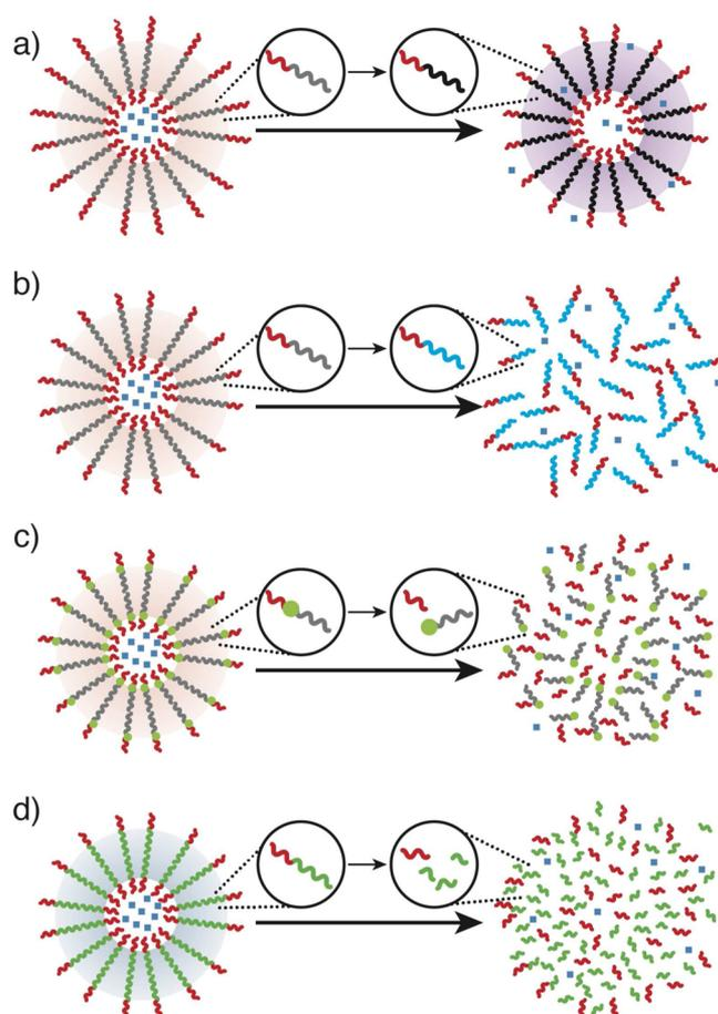
**Figure 3.** Schematic representation of triggered release from polymersomes utilizing different triggering mechanisms: (a) change in membrane permeability, (b) change in polymer polarity, (c) cleavable linkers between blocks of diblock copolymers, and (d) degradation of the main polymer backbone.
