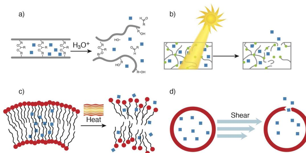
**Figure 1.** Example mechanisms of triggering. (a) pH-induced hydrolysis of an acid-labile cross-linker; (b) photolysis of photocleavable linkers in a polymer matrix; (c) thermal destabilization of a bilayer membrane by heat; (d) shear-induced cracking of an encapsulant shell.
