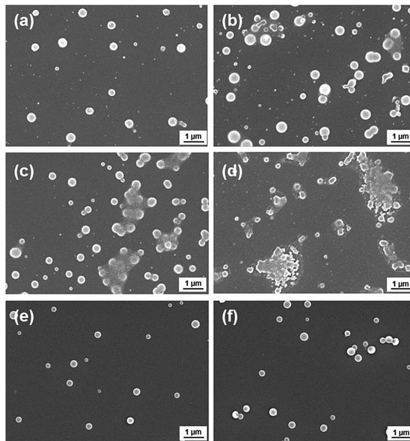
**Figure 3.** Scanning electron micrographs of NP3s (PBAE:PEG-PLA = 75:25) irradiated by UV (10 mW · cm<sup>-2</sup>) for 0 h (a), 0.5 h (b), 2 h (c), and 3 h (d), and NP6s (100% PEG-PLA) before (e) and after irradiation for 3 h (f).
