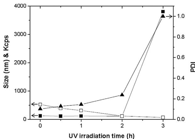
**Figure 4.** Size, kilo count per second (Kcps, light scattering intensity), and polydispersity index (PDI) of NP3s (PBAE:PEG-PLA = 75:25) as a function of irradiation time of UV ( $10 \text{ mW} \cdot \text{cm}^{-2}$ ). Arrows indicate the corresponding y-axis to size (■), Kcps (▲), and PDI (□) data.
