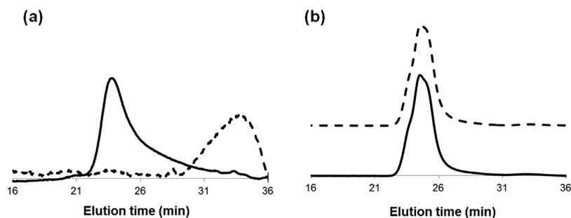
**Figure 2.** The GPC trace of the PBAE and PEG-PLA in DMF (10 mg · mL<sup>-1</sup>) as a function of UV irradiation time (20 mW · cm<sup>-2</sup>). The GPC curves for (a) PBAE before (solid) and after UV treatment for 60 min (dashed) are represented. (b) PEG-PLA before (solid) and after irradiation for 60 min (dashed) are also represented.
