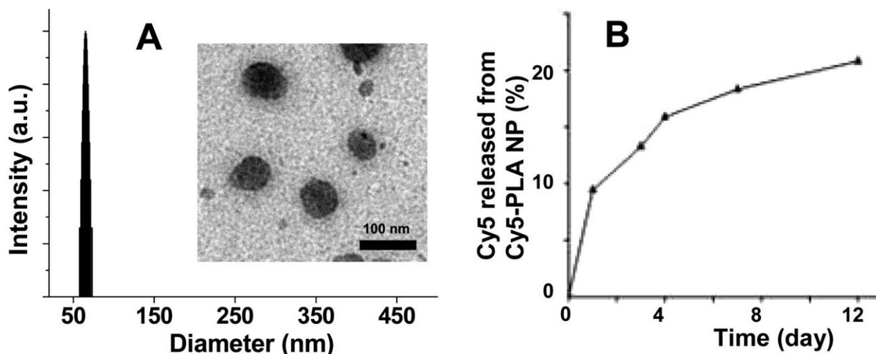
Fig. 3. Characterization of Cy5-PLA/PLA-PEG-mPEG nanoparticles by dynamic light scattering (DLS) (A) and transmission electron microscopy (TEM) (Inset). B: Release kinetics Cy5 from Cy5-PLA NP in PBS at 37°C.
