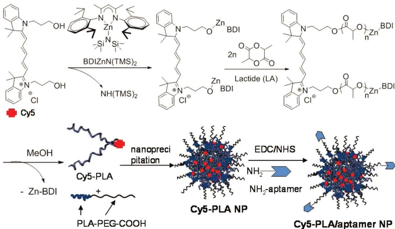
Fig. 2. Preparation of Cy5-PLA/aptamer nanoparticles via Cy5 initiated LA polymerization in the presence of (BDI)ZnN(TMS)<sub>2</sub> followed by nanoprecipitation with poly(lactide-*b*-methoxylated PEG
