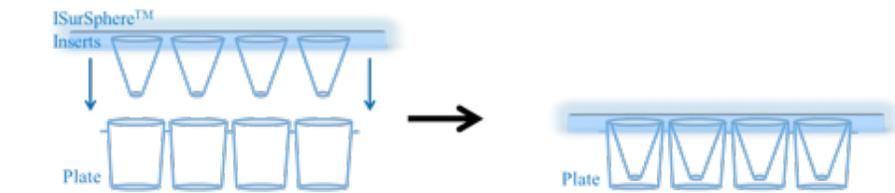
Figure 1. Schematic of a tray of conjoined ISurSphere™ inserts fitting into a 96-well plate for 3D cell culture.
