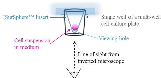
Figure 2. Schematic diagram of a single ISurSphere™ insert placed in a single well of a multi-well cell culture plate depicting a drop of cell suspension in growth medium above the viewing hole.
